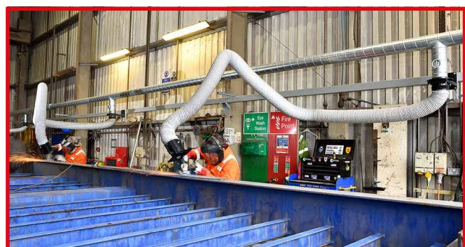
Supplied with sturdy wall bracket, flanged adaptor and hood with a built-in damper. A halogen lamp cartridge can be fitted to the hood as an optional extra. Our Flexi Arm 5.0 metre is also available in 200mm dia.
